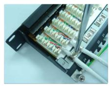
Fasten the screws through metal case to hold tightly down for two cable jackets in the same time.
